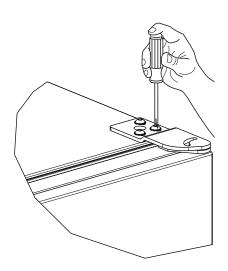
Remove door by tilting forward and lifting door off bottom hinge. Retain shoulder washer; it will be reused.
