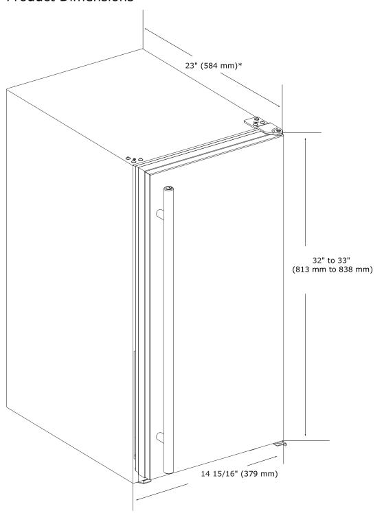
\*Add 3/4" To Depth For Water Line Clearance
