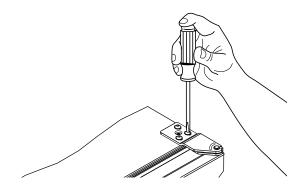
3. Remove door by tilting forward and lifting door off bottom hinge. Retain shoulder washer; it will be reused.
