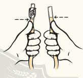
...and attach the non-clamped end to the racking cane; this will be your siphon starter.
