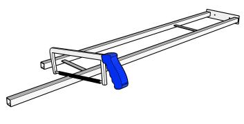
3. Assemble the frame - Slide the frame together with the couplers aligning the two sections. Secure the WS-Series racks and/or FCF-BACK to the the front and back faces, ensuring that the coupled joint of the frame is spanned by the back strip of a WS-Series rack or an FCF-BACK and that the rack or FCF-BACK spanning the joint is screwed into both the upper and lower sections of the frame (Inset A).
