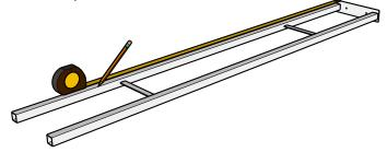
2. Cut the frame - Using a metal cutting saw, squarely cut both legs of the FCF-HD to length and remove any resulting burrs with a metal file.
