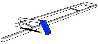
3. **Insert the FCF-BASE** - Slide the FCF-BASE into the newly cut end of the FCF-HD and use this end as the top of the frame.
