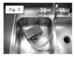
sanitizing solution as previously described. Drain and allow to drip-dry. Do not store the unit full of sanitizer due to potential galvanic corrosion issues. An alternate method to sanitize the unit is to immerse it in boiling water for 10-15 minutes, which will completely sterilize it.
