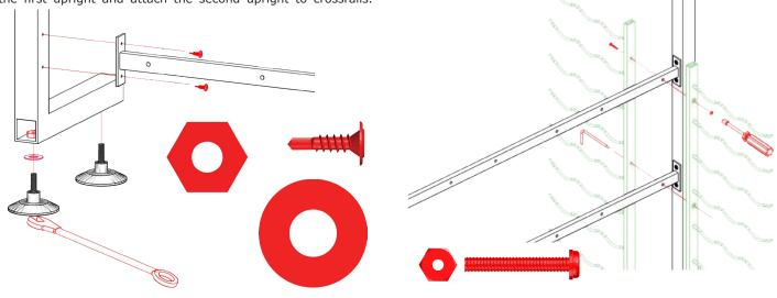
3. **Assemble presentation rack** – Position presentation rack (IDR-PR) piece and presentation rack rail (IDR-H-PRR) back to back as shown. Using the nut driver (included) and a Phillips head screwdriver, fasten the presentation rack and rail together with IDR-PR assembly screws. Fully tighten.
