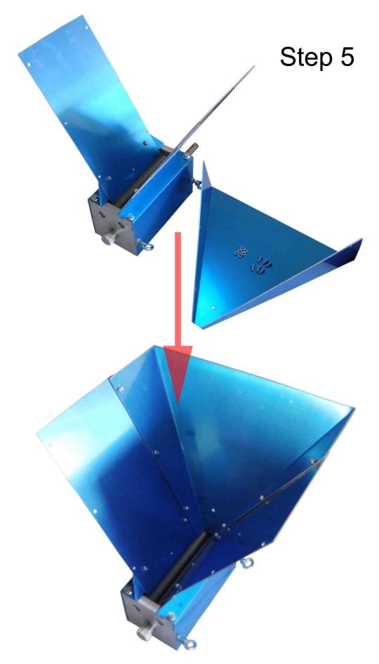
Attach the Hopper Side Panel over the top of the Hopper Front and Back Panels.
