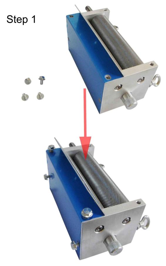
Use four of the large screws to attach the Hopper Base Panel to the Rollers Body.
