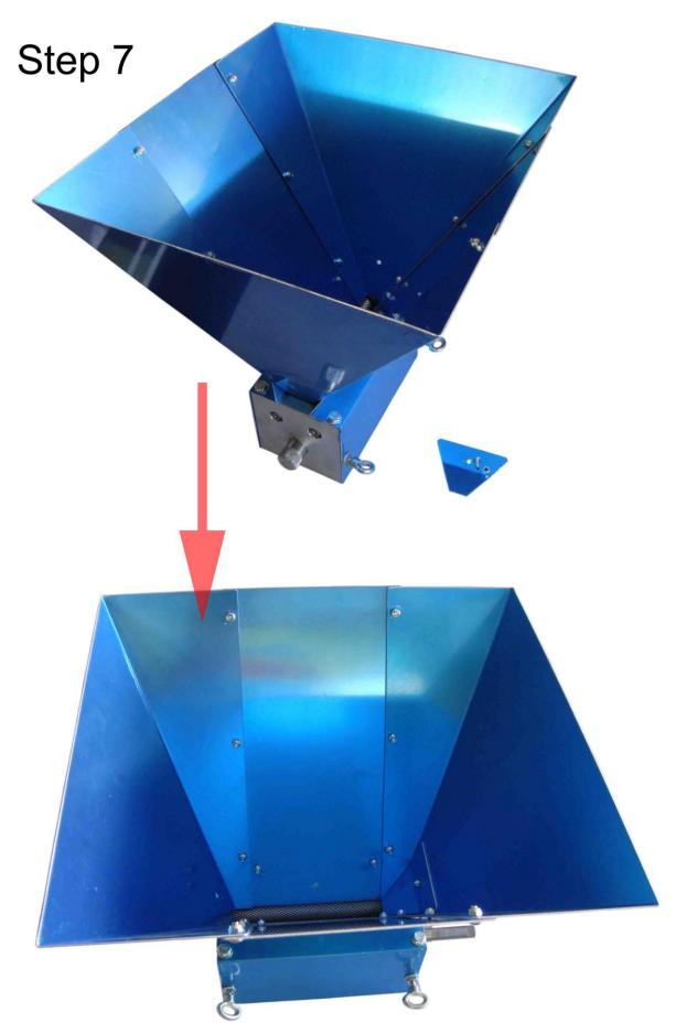
Attach the Hopper Guide Panels to the Hopper Side Panels to ensure grains are properly directed into the mill.
