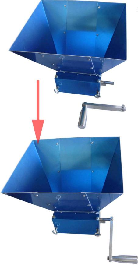
Attach the Handle to the crankshaft on the Rollers Body, ensuring that the screw tightens onto the flat portion of the crankshaft.
