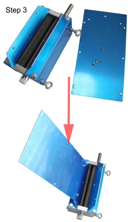
Attach the Hopper Back Panel to the Hopper Base Panel with the smaller screws and lock nuts provided. You will need a small screwdriver and pliers to hold the lock nut as you turn the screws.
