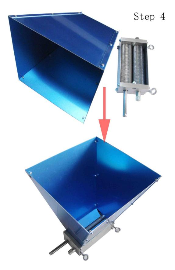
Loosen the nuts on the Rollers Body to attach the Hopper to the Rollers Body. The cut outs on the bottom tabs of the Side Panels should fit over the exposed screws. Tighten the nuts back down to fasten the Hopper in place. You may need to bend the tabs slightly to make them fit inside the Rollers Body as shown.
