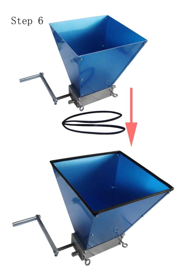
Install the Hopper Gasket around the upper edge of the Hopper Panels.
