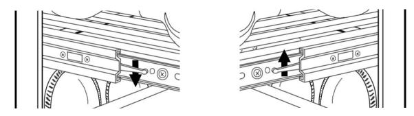
The shelves are removable to help with cleaning and maintenance. To remove a shelf, pull it out as far as you can. There are levers on each side of the shelf near the rollers. Lift the lever on the left hand side and push down on the lever on the right hand side to remove the shelf from the tracks.
