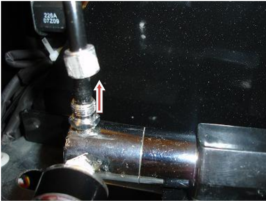
Loosen the nut tube at the top.
