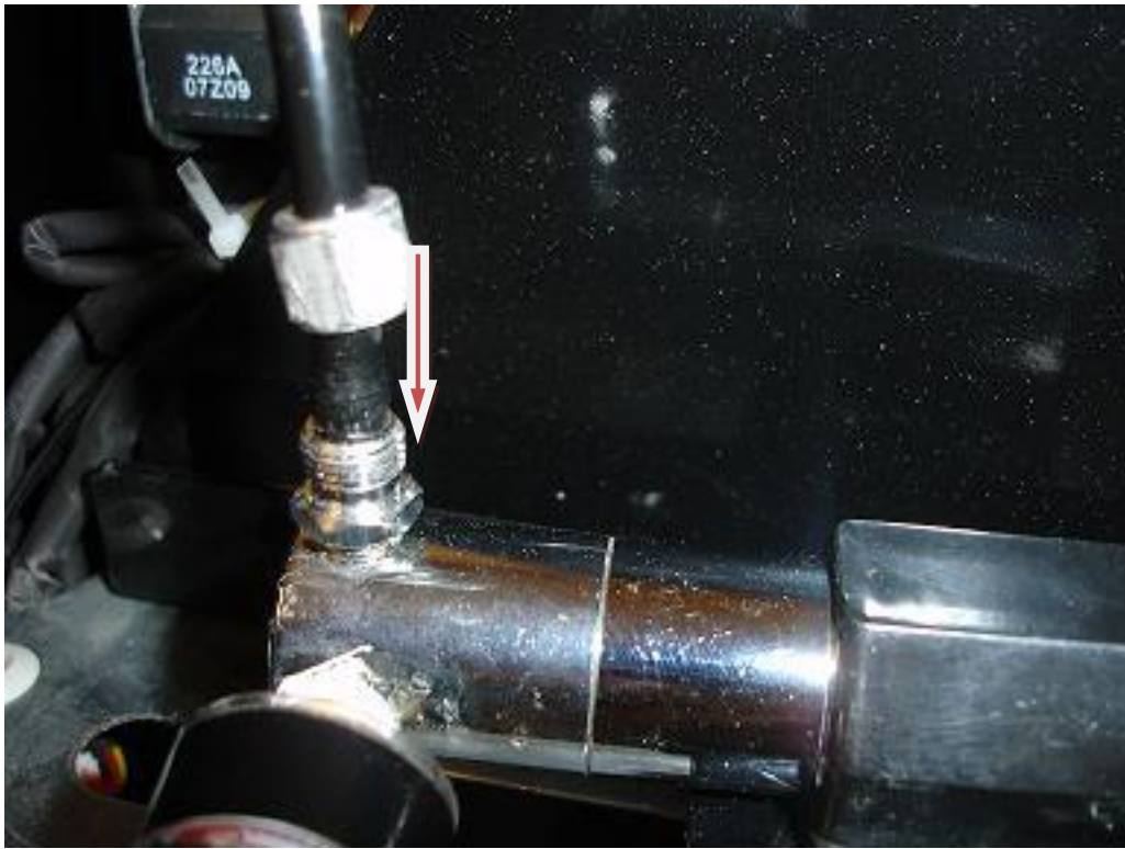
Reattach the hose to the new regulator.
