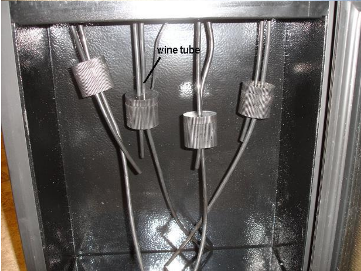
Pull and disconnect the wine tube.
