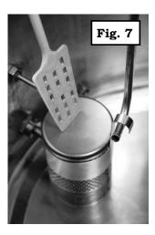
**Tip:** Allowing adequate time for the break material to settle is necessary for proper performance. In addition, draining slowly at the end is vital to allow the wort to filter through the break material and move toward the filter. If it is drained too quickly you will draw the particulates with it toward the filter and increase the likelihood of plugging it. Draining slowly allows the wort to permeate the sediment and move to the filter. At all times be careful not to disturb the sediment!
