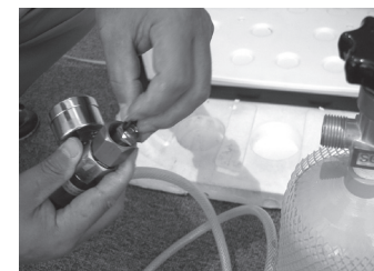
Illustration A High Pressure Washer Installed into CO 2 Regulator
