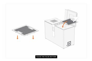
Place the false bottom into the mashing tank, legs straight at the bottom of the tank.
