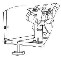
Break away filler feature in bushing with flat screwdriver.
