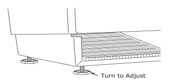
3. Confirm the unit is level after each adjustment and repeat the previous steps until the unit is level.
