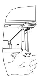
4. Remove four screws from hinge holes on the opposite side. Reinstall into holes where the hinge was removed. Take care not to scratch cabinet.
