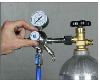
will start to pour. Stop turning when you get the best flow rate. This should be in between 8 and 10 PSI. This method should prevent your regulator from creeping.
