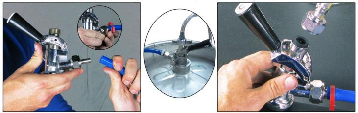
Home Brew Couplers - Home brew couplers have a separate attachment for the gas in and liquid out. The air tube attaches in the same manner as the commercial coupler. The liquid out home brew coupler uses a hose nipple so you must cut off the fitting on the end of the beer line to attach it to the liquid out coupler. Clamp each hose into place.
