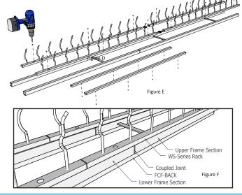
For product warranty information, please visit: <u>www.VintageView.com/support/warranty</u> We're here to help, call us at 866-650-1500 with any questions. 5. **Insert the mounting plates** - Slide the C-channels of the base mounting plate(s) into the bottom of the frame, ensuring that the frame is seated flush against the horizontal plate. Then, install the wall brackets, and secure both sets with a self-drilling screw through the side of the frame.
