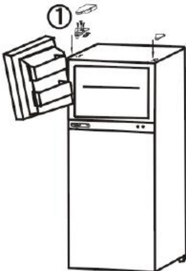
Place the freezer door on the middle hinge. Ensure that the door is aligned horizontally and vertically, and that the gasket seals on all sides before attaching the top hinge. Attach the top hinge and replace the hinge cover.
