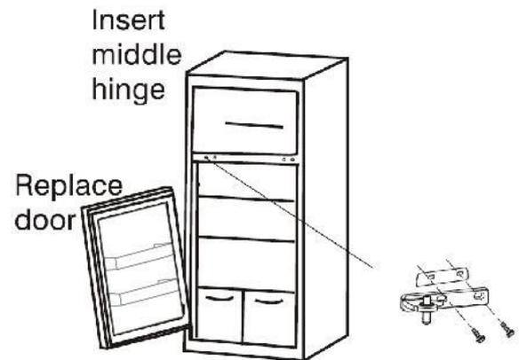
Place the refrigerator door on the bottom hinge. Be sure the door is aligned horizontally and vertically. Attach middle hinge to refrigerator door and attach bolt washer to the back of the hinge, then fix them to middle beam and fasten them with a screwdriver.
