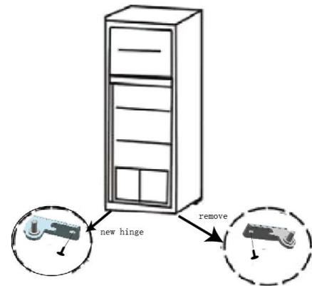
Remove right bottom hinge and reserve the screws. Remove screw covers at left corner and put them into the screw holes at right corner. Install left hinge by using those reserved screws.
