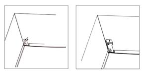
13. Place the top left cover on the right side and fix it by using the screws.
