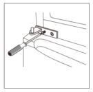
12. Place the upper door back onto the unit. Ensure the door is aligned horizontally and vertically so that the seal is closed on all sides before finally tightening the top hinge. Then insert the top hinge and screw it to the top of the unit and then the affix hinge cover (in the accessory bag) by using the screws.
