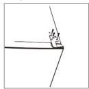
Remove the pin with a screwdriver and flip the hinge bracket. Then refit the pin to the hinge bracket.
