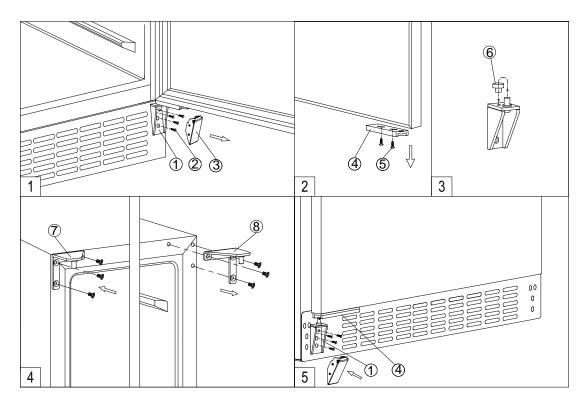
**NOTE:** All parts removed must be saved to allow the door swing to be reversed.
