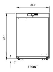
\*For Built-In Applications: Allow 1.2" (30mm) at top for stainless steel louvered vent.
