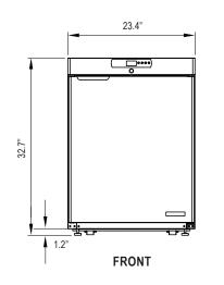
\*For Built-In Applications: Allow 1.2" (30mm) at top for stainless steel louvered vent.
