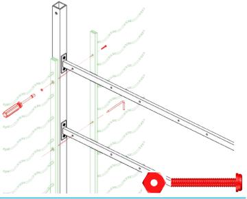
3. **Assemble presentation rack** – Position presentation racks back to back as shown. Using nut driver (included), a Phillips head screwdriver (not included) attach presentation racks with presentation rack assembly screws. Fully tighten.
