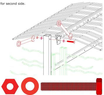
5. **Finishing steps** – Fully tighten all screws (especially Crossrail Assembly Screws) and snap mounting hole covers in place. Fill with wine and enjoy!
