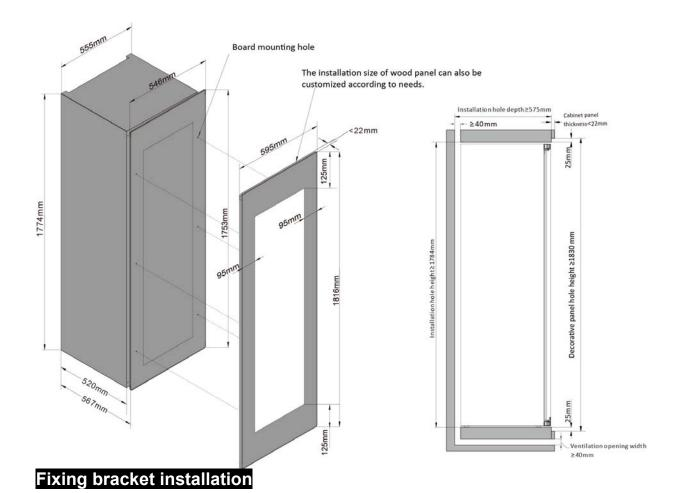
1.Level the wine cooler, take 2 fixing brackets ①  $2 \times 5*16$  flat head screws ② and 4 screw covers ③ from the polybag. Remove 4 trunk-nails on the left side frame, fix the brackets ① on the left side of with a philips screwdriver.
