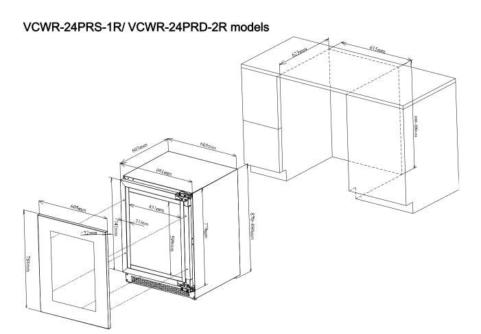
After adjusting the door panel, take out 4pcs 5\*35 self-tapping screws from the accessory bag, open the door seal, drill the screws through the screw holes in door frames, and tighten the door panels.
