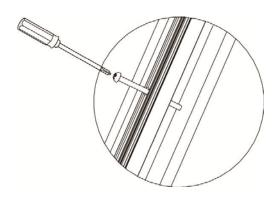
1.Level the wine cooler, take 2 fixing brackets ①  $2 \times 5*12$  flat head screws ② and 2 screw covers ③ from the polybag. Remove 4 trunk-nails on the left side frame of cabinet, fix the brackets ① on the left side of canbinet with a philips screwdriver.
