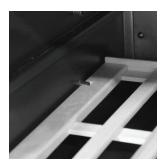
With the notches and stoppers still lined up, push down on the front of the shelf and the shelf will lift up past the stoppers.
