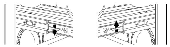
You can remove a shelf to accommodate larger diameter bottles on the shelf below it. To remove a shelf, pull it out as far as you can. There are levers on each side of the shelf near the rollers. Left the lever on the left hand side and push down the lever on the right hand side to remove the shelf from the tracks.
