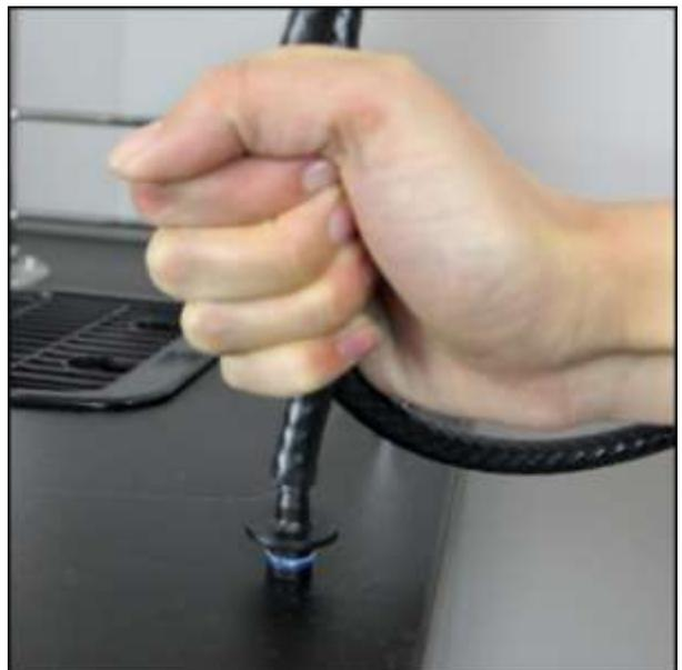
Insert Plastic Hose Barb (4) into Plastic Tube, pressing firmly until the flat portion touches the end of the hose. Use a hard surface to press down, if necessary.
