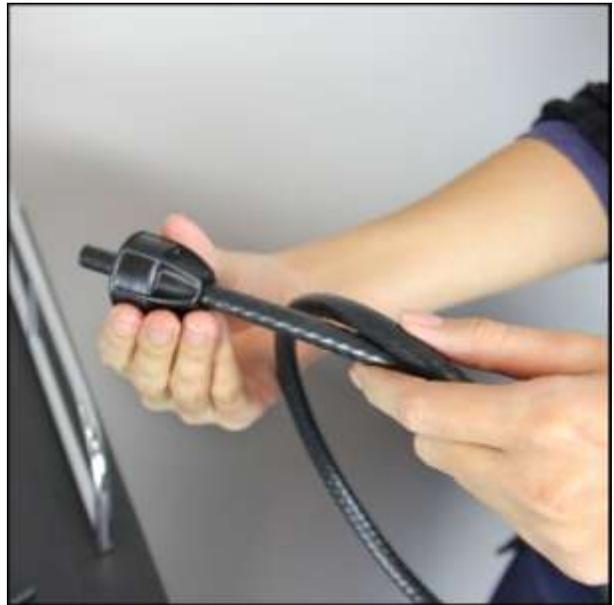
Slip plastic screw cap (7) onto 3/16" I.D. Plastic Tube (9), ensuring the flared end (larger opening) faces outwards.
