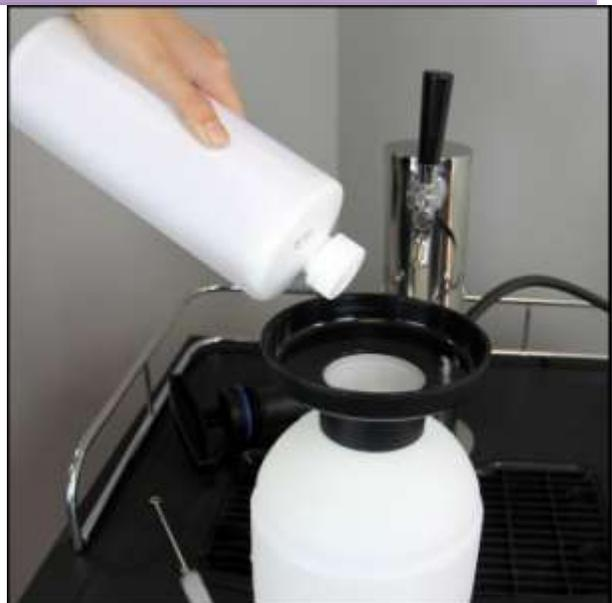
Attach the beer line to the Duplex Coupler. Pour the measured amount of the Cleaning Chemical (10) into the open Cleaning Bottle, following the manufacturer's specifications on the label. Add water as directed, ensuring not to overfill the container.
