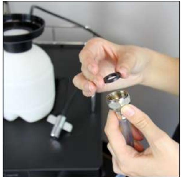
Make sure to keep the Neoprene Washer (9) in between the beer line fitting and the Duplex Coupler.
