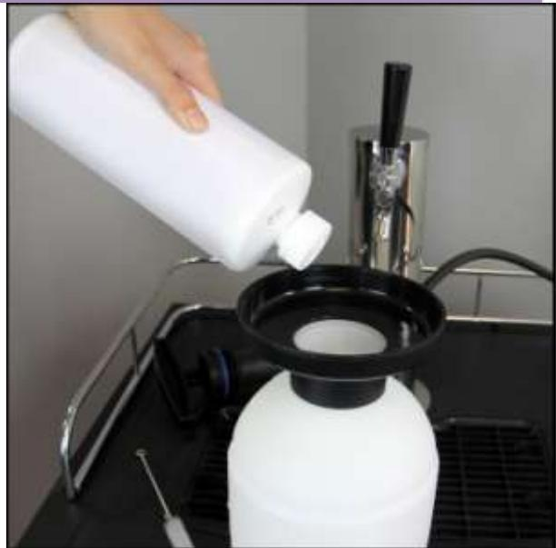
Attach the beer line to the Duplex Coupler. Pour the measured amount of the Cleaning Chemical (8) into the open Cleaning Bottle, following the manufacturer's specifications on the label. Add water as directed, ensuring not to overfill the container.
