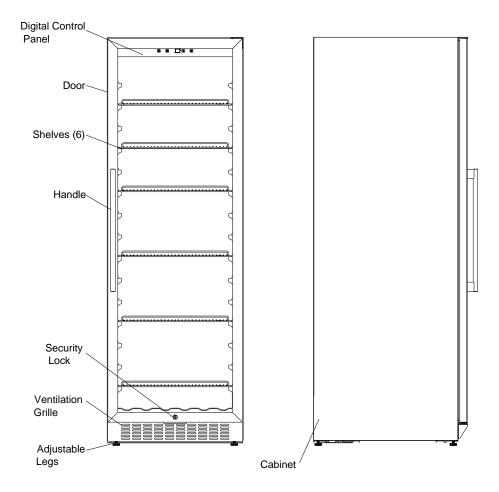
\* NOTE: Model SCR1400WLH opens from the right, so handle is on that side.
