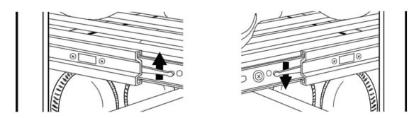
The shelves are removable to help with cleaning and maintenance. To remove a shelf, pull it out as far as you can. There are levers on each side of the shelf near the rollers. Lift the lever on the left hand side and push down the lever on the right hand side to release the shelf from the tracks.
