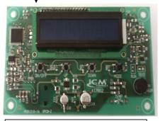
**Local User Interface**: Can be used with Main Control for adjusting settings, reading temp/humidity, and reading fault codes at the unit.
