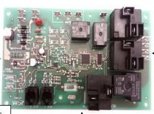
Two way communications: local user interface reports settings back to main control, main control energizes outputs and reports alarms and temp/humidity readings to local user interface.
