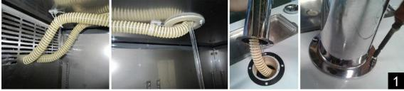
1. Insert the air hose into the beer tower and secure the beer tower to the cabinet with the gasket under the beer tower.
