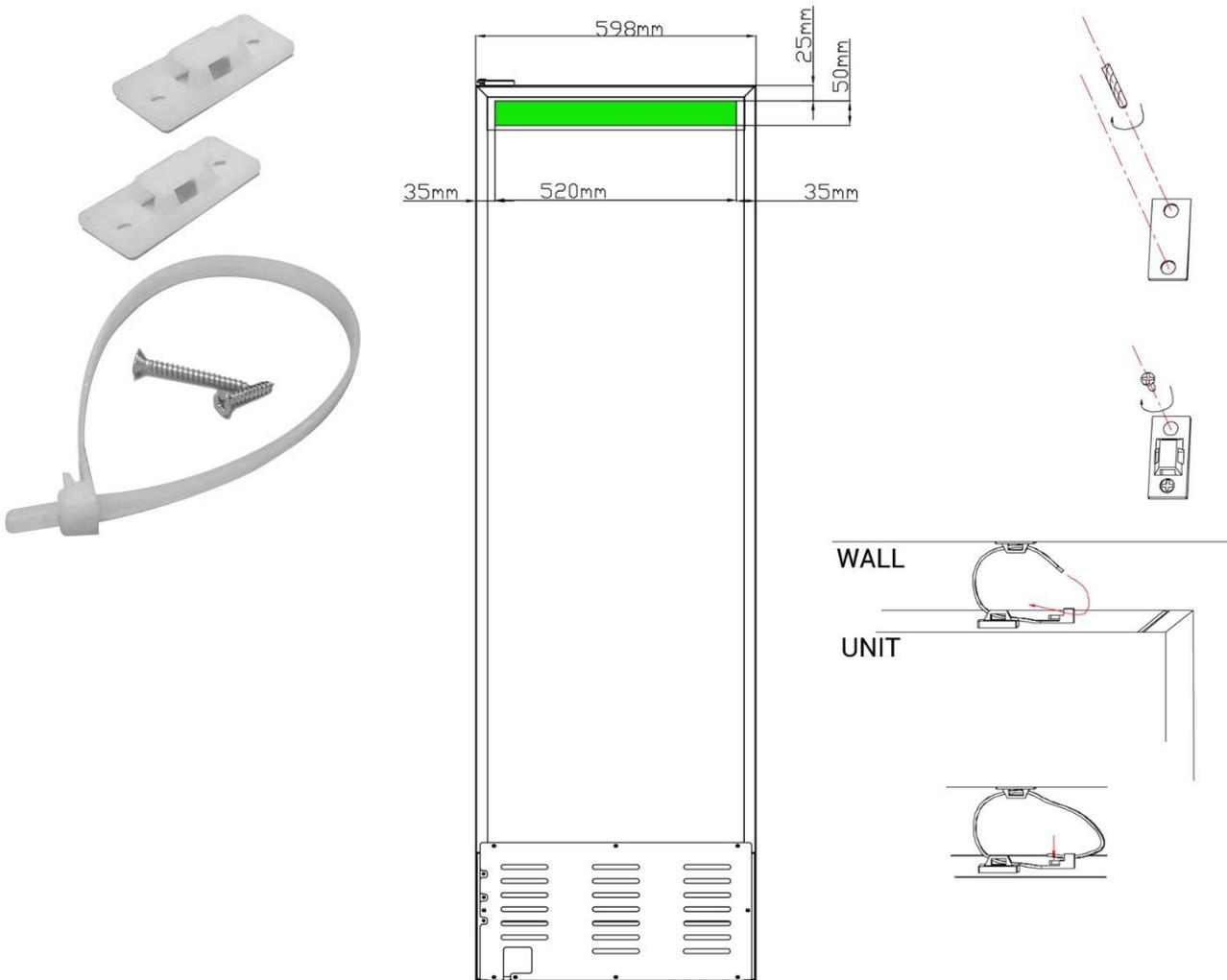
1. On the back of the appliance, attach brackets in the same zones shown using adhesive straps. Mark and drill pilot holes for the screws about 8mm into the appliance. Then use a screwdriver to tighten the screws all the way into the appliance.
