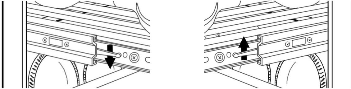
You can remove a shelf to accommodate larger diameter bottles on the shelf below it. To remove a shelf, pull it out as far as you can. There are levers on each side of the shelf near the rollers. Left the lever on the left hand side and push down the lever on the right hand side to remove the shelf from the tracks.
