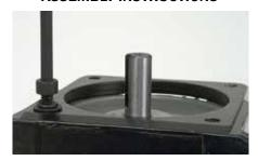
1. Install the motor mount on the motor/gear box assembly with the four 5mm hex key screws and washers so the wire comes out the top when finished. The motor can also be installed so the wire comes out on the bottom, but then you will have to shim up the Mill a ¼" or so off the base to align with the motor shaft (we have found it is easier to shim up or down
